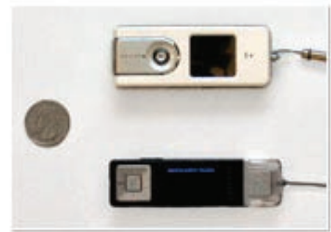
The Go Meters identify viewing by collecting audio signatures (MP3-based and cell phone-based).
